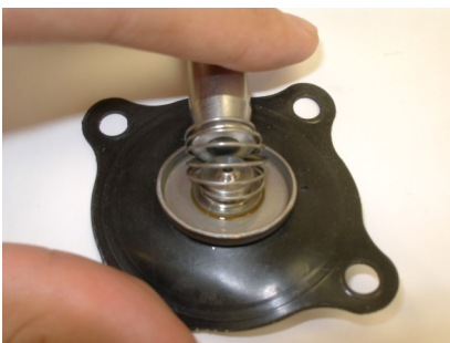
Figure 4: Complete assembly of direct lift diaphragm valve
